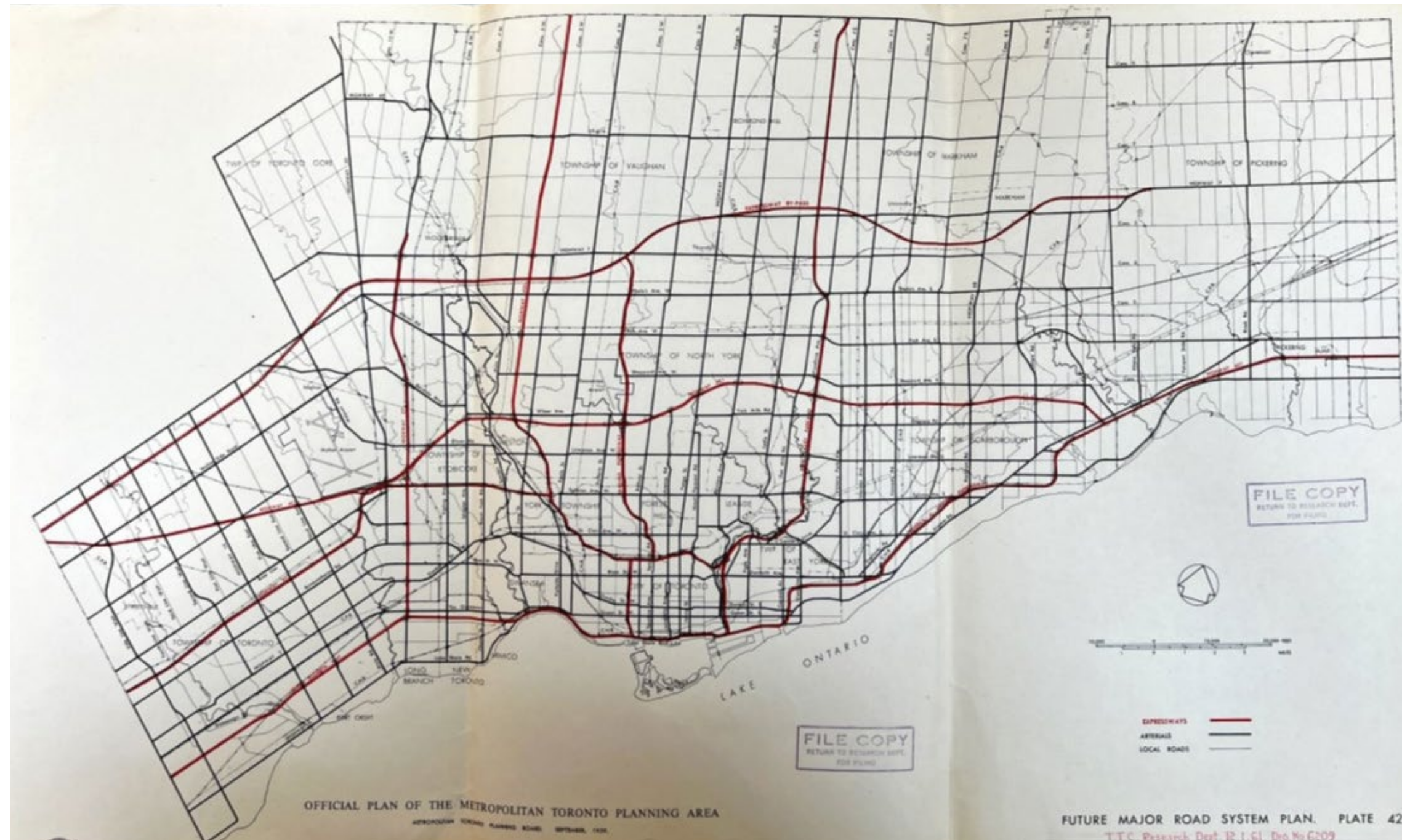
Figure 4 : Future Major Road System Plan, Official Plan of the Metropolitan Toronto Planning Area. Expressways are marked in red, arterial roads in black 47
